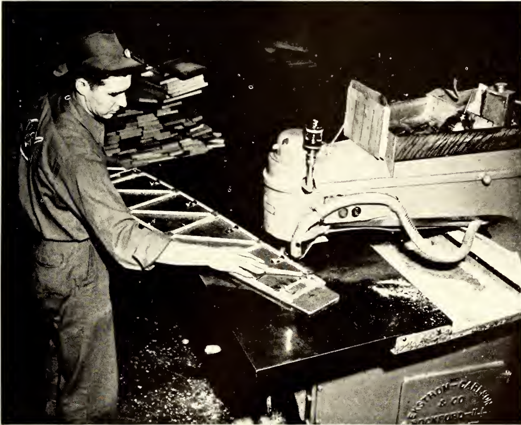
FIGURE 5-82.—Routing wing ribs to contour.
